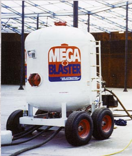
Trailer mounted Mega Blaster with 4 outlets on large water tank project. Holds enough Garnet to Blast all day without stopping.
